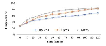
FIG. 5: Temperature difference in solar cooker with different number of convex lens.
