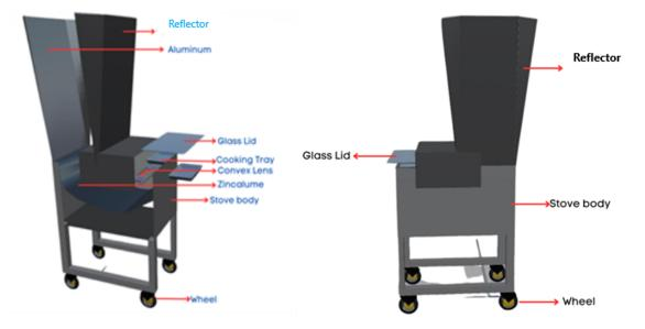
FIG. 1: Solar cookers with convex lens addition.
