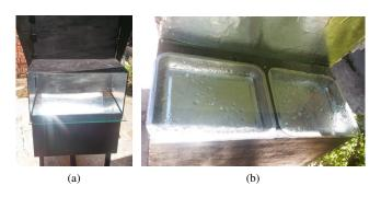
FIG. 4: (a) Solar radiation in solar cooker without cooking tray, (b) Water heating with solar cooker
