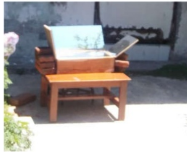
Figure 3. Solar cooker box type with mirror reflector in a back yard.
