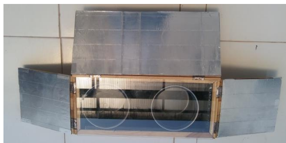
Figure 2. Solar cooker box type with Aluminum Tape reflector
